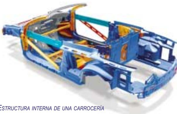
ESTRUCTURA INTERNA DE UNA CARROCERÍA
